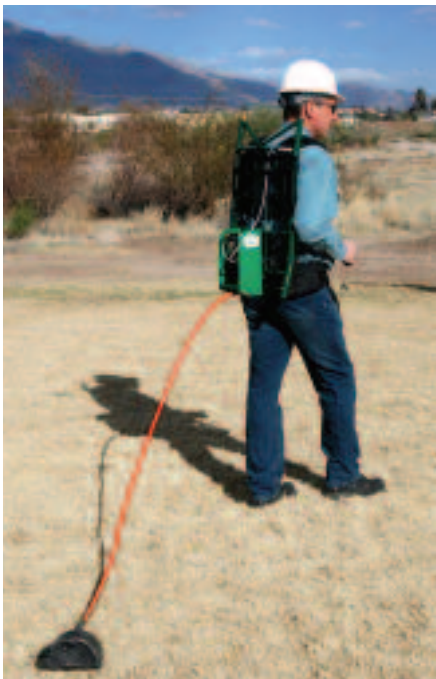
The unique Seeper Trace leak detection method utilizes an active sampling device to collect representative sub-surface soil gas from the ground surface without disturbing or penetrating the ground.
